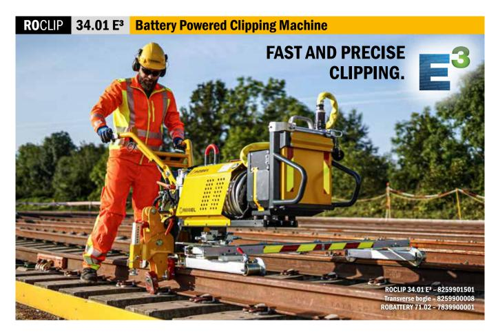
For emission-free inserting and extracting Fastclip clip fasteners in new construction and maintenance. With sleeper lifting unit.
